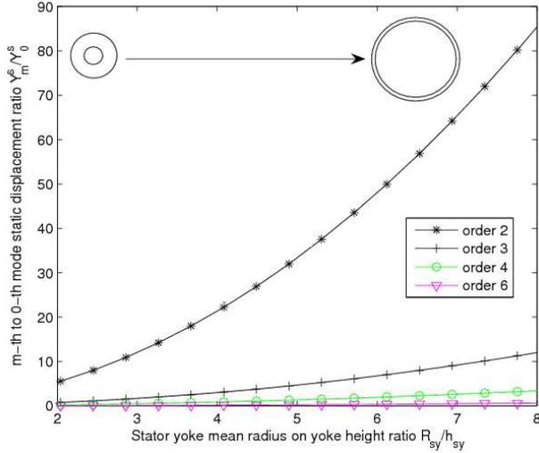
Fig. 4. Relative static displacement in function of  $R_{sy}/h_{sy}$  ratio for several modes. Doubling the relative static displacement increases the sound power level at resonance of  $10 \log_{10}(2^2) \approx 6$  dB.
