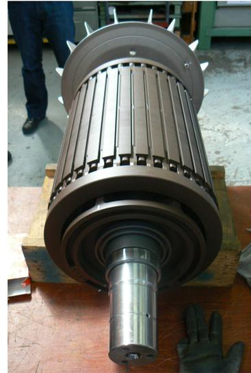
Fig. 11. New rotor of the industrial 250 kW motor.
