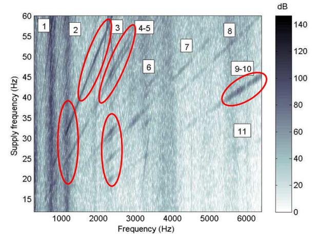
Fig. 9. Simulated (top) and experimental (bottom) acceleration spectrogram in sinusoidal case (laboratory motor,  $f_s=12$  to 60 Hz). An uncertainty exists on the experimental supply frequency as no tachometer probe could be used.
