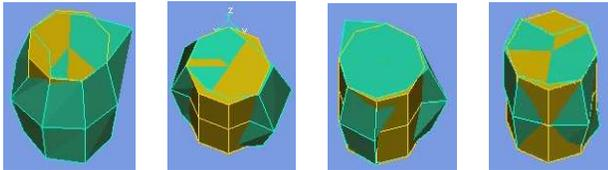
Fig. 8. Deflection shapes of some stator circumferential modes of the laboratory motor ( $m = 0$ : breathing mode,  $m = 2$ : elliptical mode,  $m = 3$ : 3-order elliptical mode,  $m = 4$ : 4-order elliptical mode).
