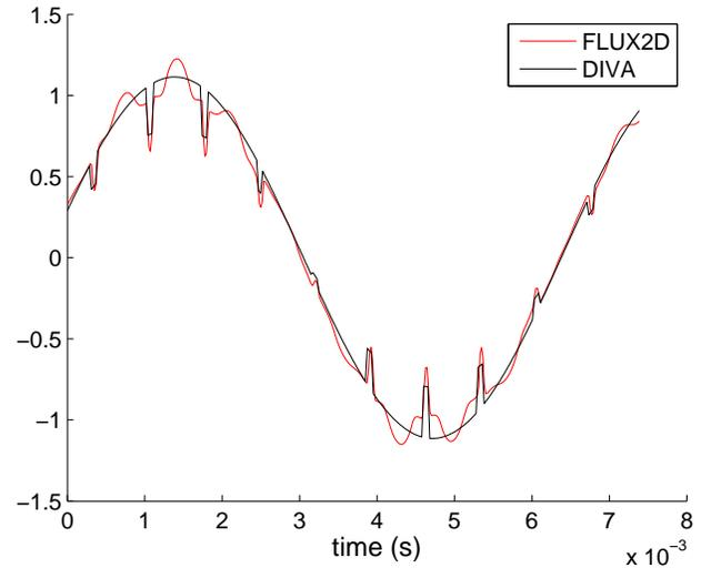
Fig. 5. FEM and analytical radial flux density distribution along the air-gap (top) and in function of time (bottom) (sinusoidal no-load case).
