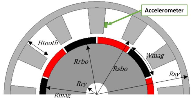
Fig. 1. Prototype 12S10P SPMSM for experimental validation
